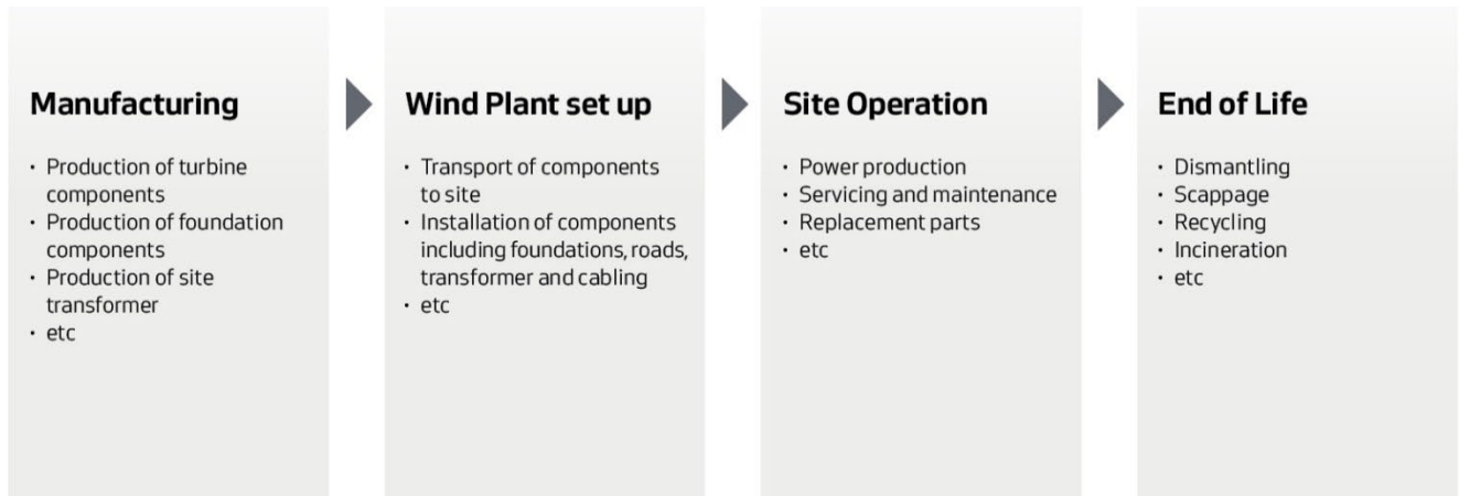
Figure 4: Life cycle stages of a typical onshore wind plant including typical activities
