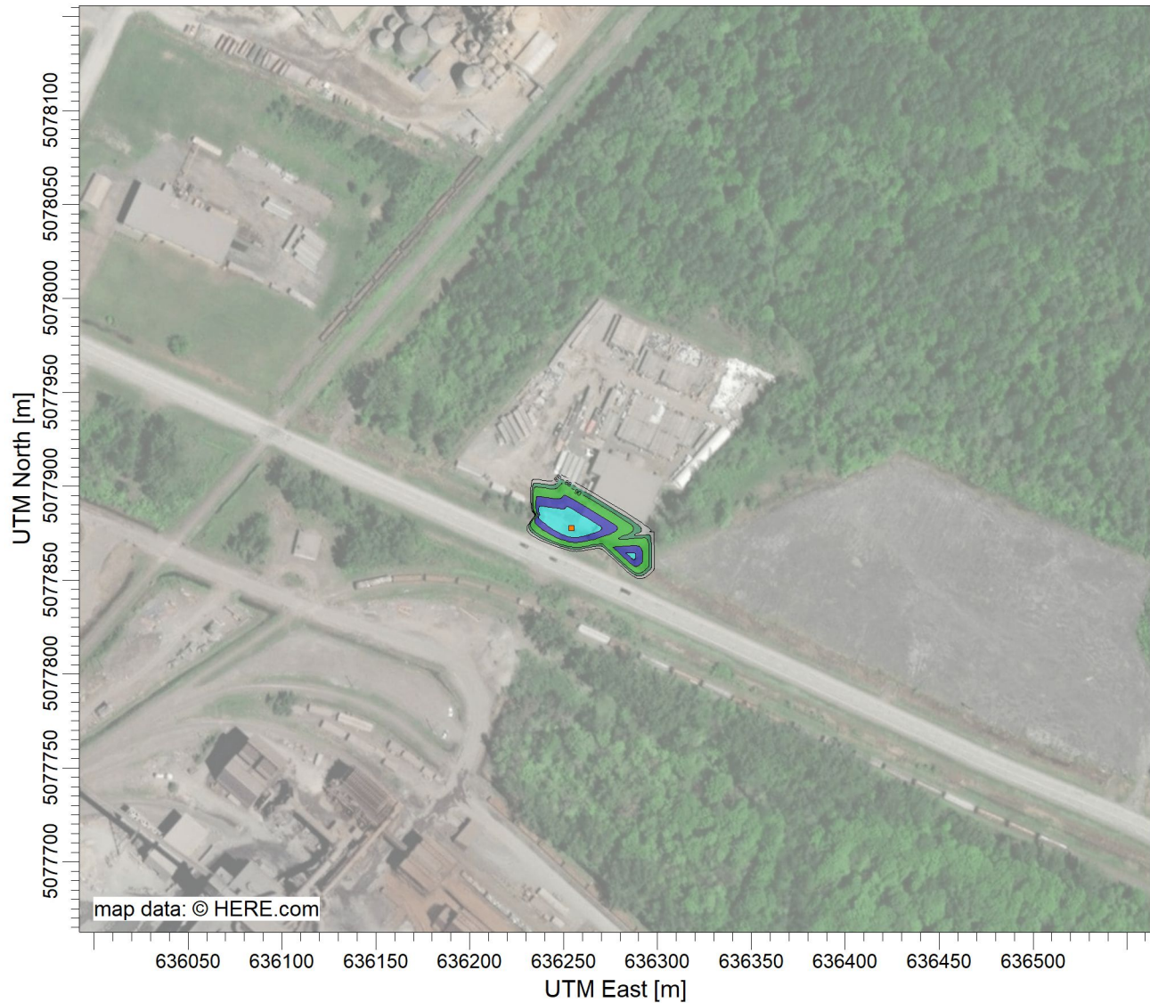
PLOT FILE OF HIGH 1ST HIGH 1-HR VALUES FOR SOURCE GROUP: ALL ug/m^3 Max: 110 [ug/m^3] at (636254,37, 5077877,51)
