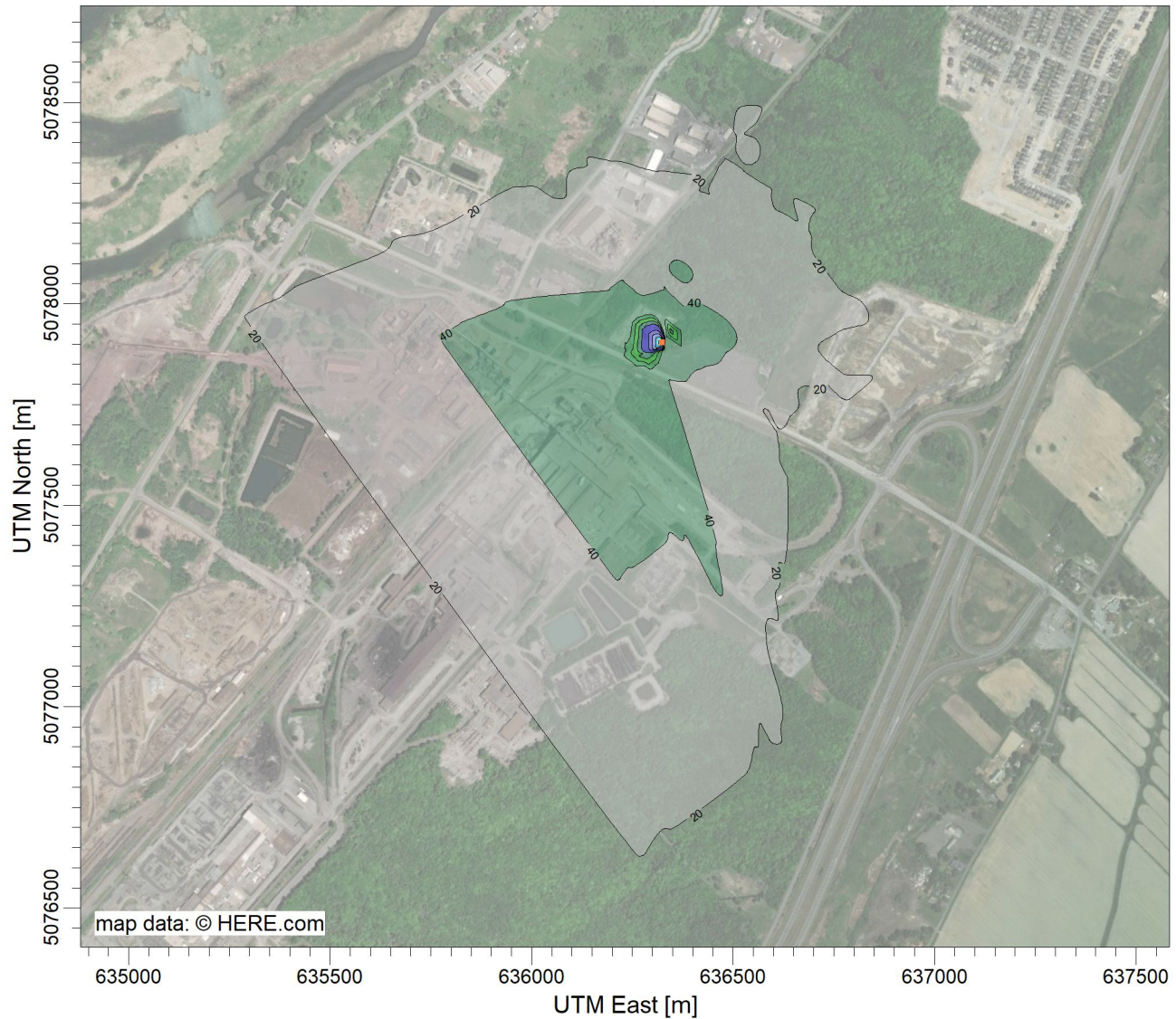
PLOT FILE OF HIGH 1ST HIGH 1-HR VALUES FOR SOURCE GROUP: ALL ug/m^3 Max: 256 [ug/m^3] at (636322,59, 5077903,65)
