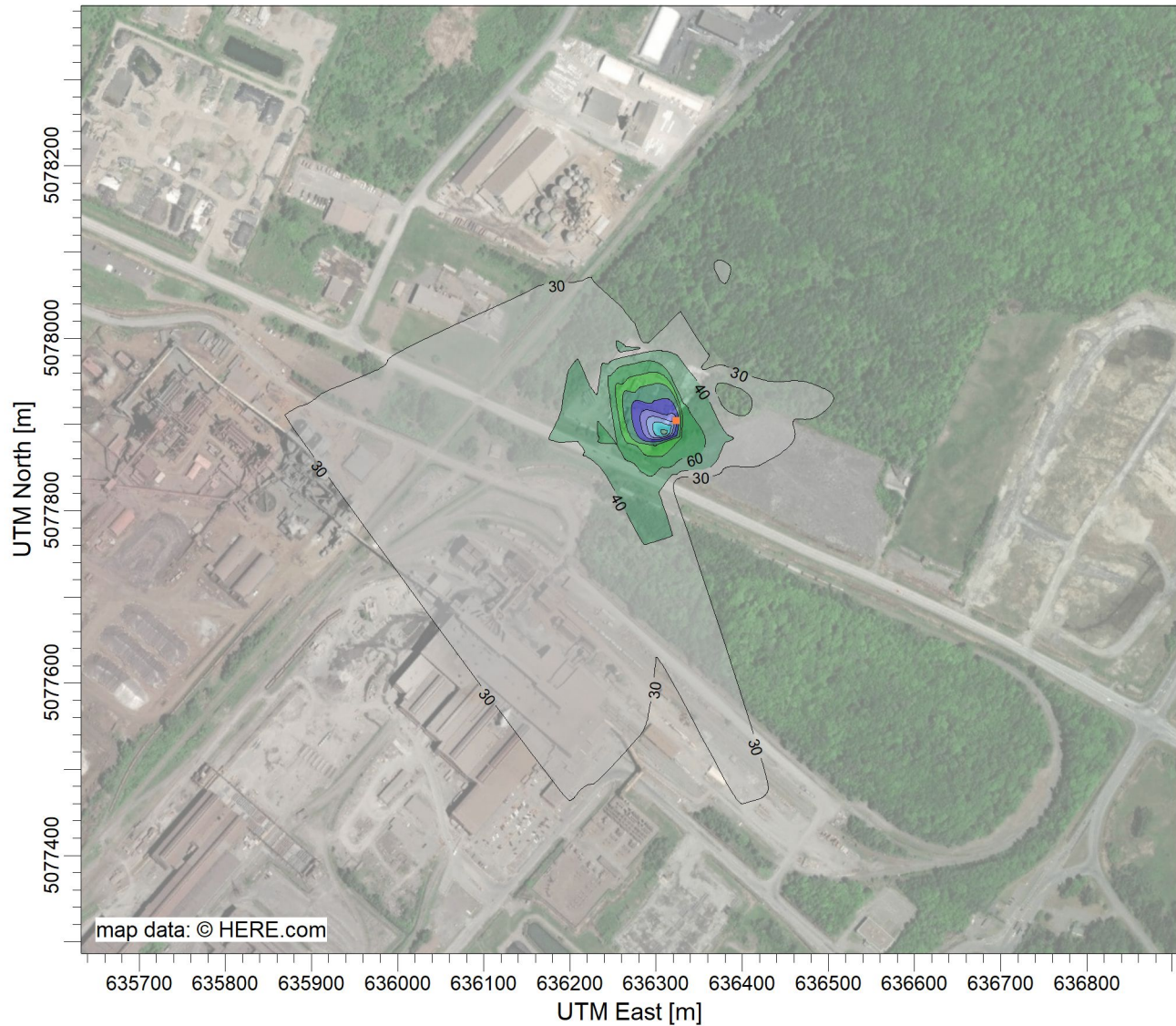
PLOT FILE OF HIGH 1ST HIGH 1-HR VALUES FOR SOURCE GROUP: ALL ug/m^3 Max: 321 [ug/m^3] at (636310,63, 5077890,02)
