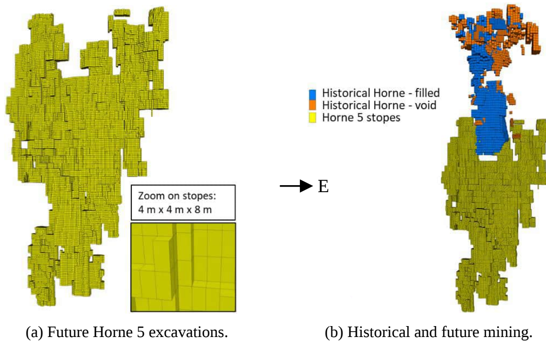
Figure 2. Views of the inside FLAC3D geometry.
