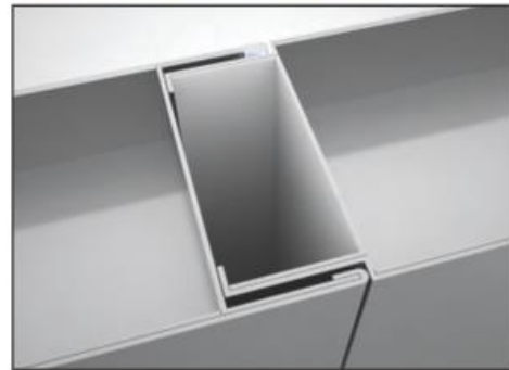
Typical groove and tongue (GT) panel joint
