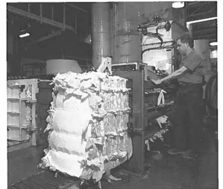
Polyethylene cut-outs that have been recovered and compacted are sold to a plastic products manufacturer.
