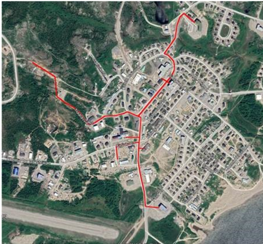
Figure 18 - Map of Kuujuaq with district heating connections (basis model) 2 MW heat demand
