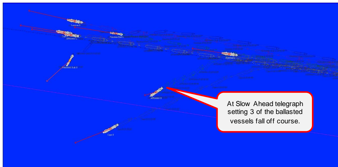
Figure 74: JDF TSS Heading Holding Test 10 Group 2 Wind 143° Slow Ahead Track-plot
