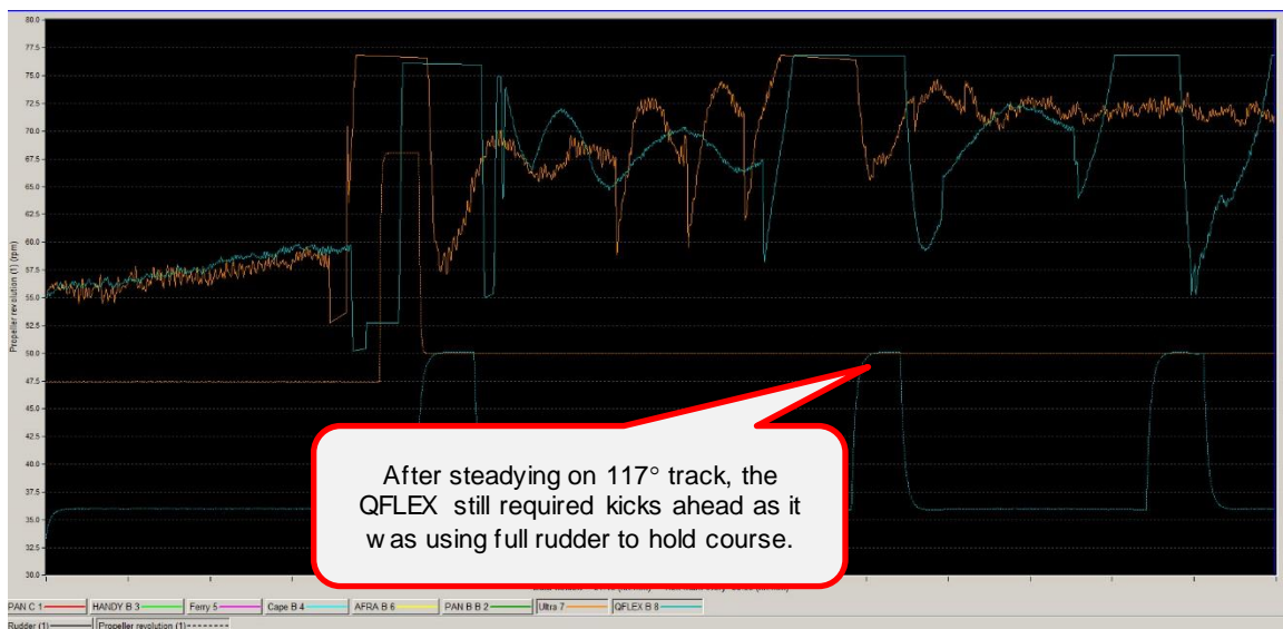
Figure 105: Anticosti Test 3 – RPM and rudder Graph QFLEX and Ultra Large Cruise
