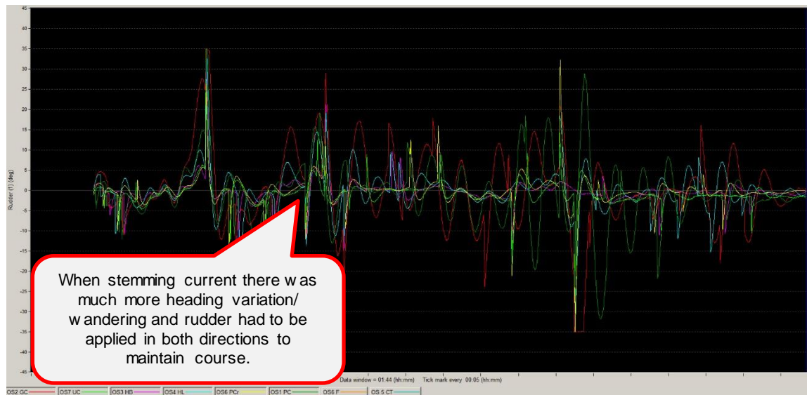
Figure 112: Test Group 1 Applied Rudder Graph: Upriver with Maximum Ebb
