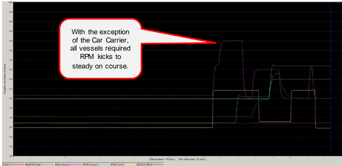
Figure 140: Rounding Turn Point - Flood Tidal Stream propeller RPM Test G1 T4
