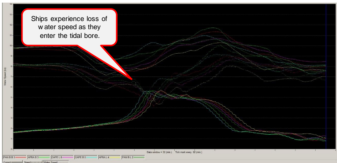
Figure 143: Speed Loss Due to Drift – East Point Southbound Test G2 T8 Speed Graph
