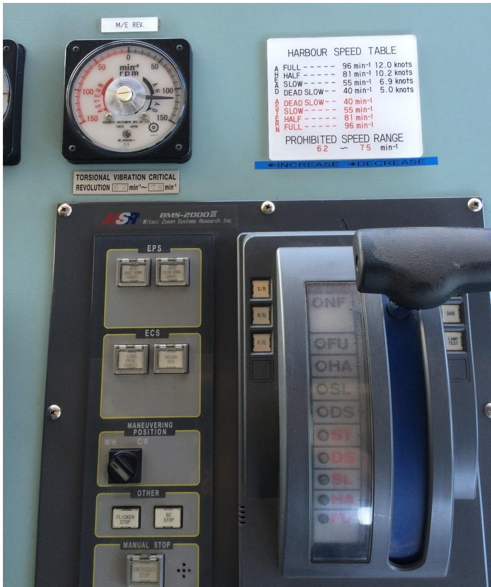
Figure 17: Sample Engine Telegraph and RPM Speed Table
