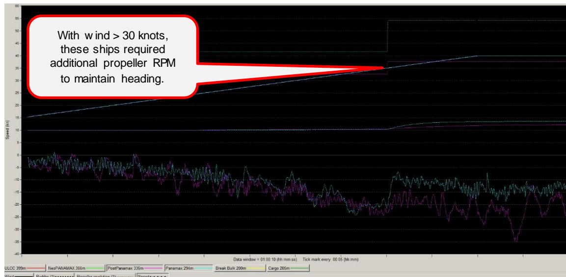
Figure 71: JDF TSS Heading Holding Test 16_2 Group 1 Wind 143° Rudder/RPM/ Vessel Speed/Wind Speed Comparison PANAMAX and Post-PANAMAX
