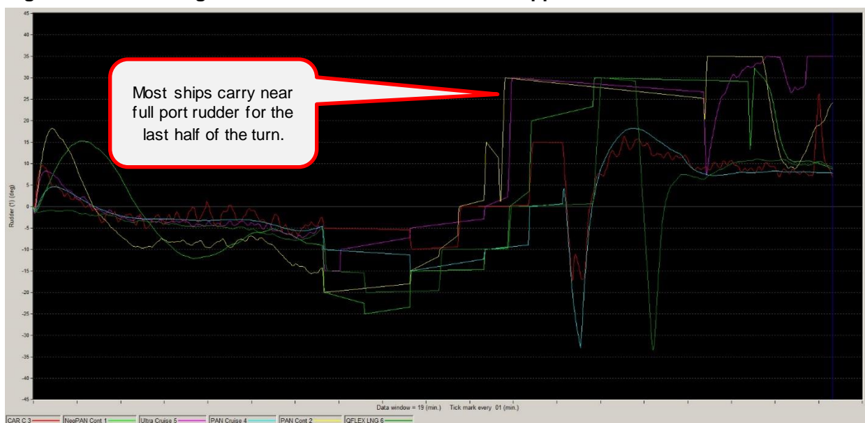
Figure 139: Rounding Turn Point - Flood Tidal Stream Applied Rudder Test G1 T4
