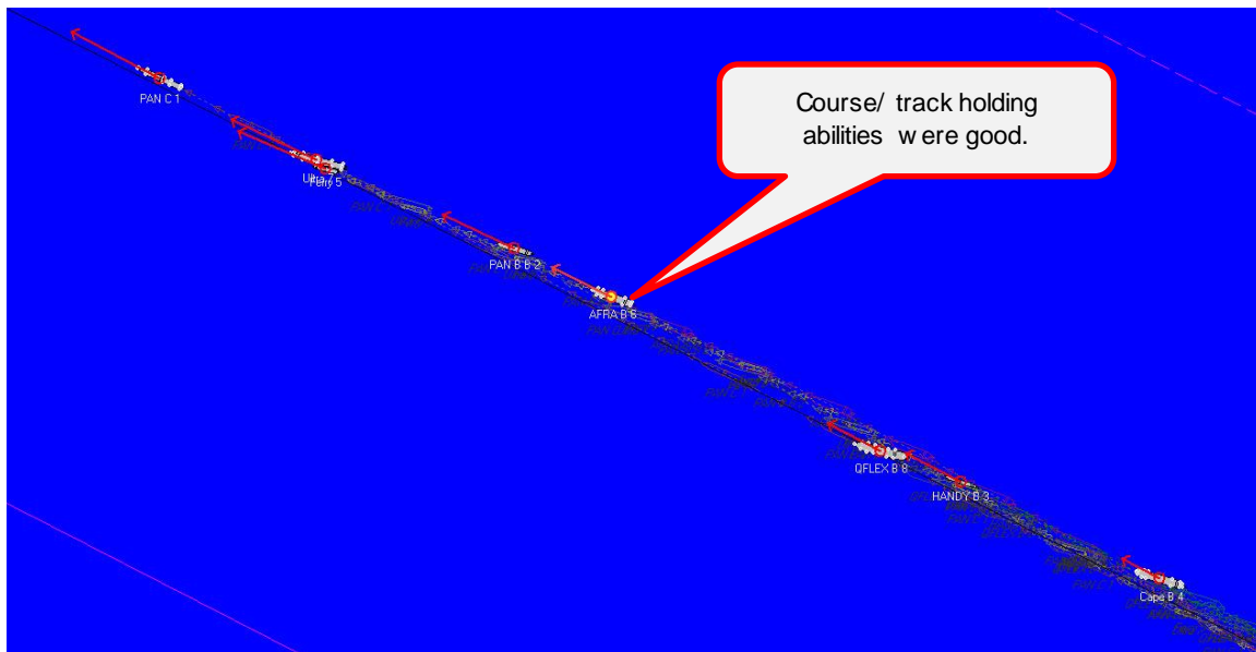
Figure 99: Anticosti Test 1 Trackplot – Wind on Bow, Constant Propeller RPM at Slow Ahead
