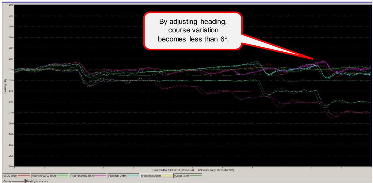
Figure 61: JDF TSS Heading Holding Test 9-1-Group 1 Wind 247° Heading and Course Graph
