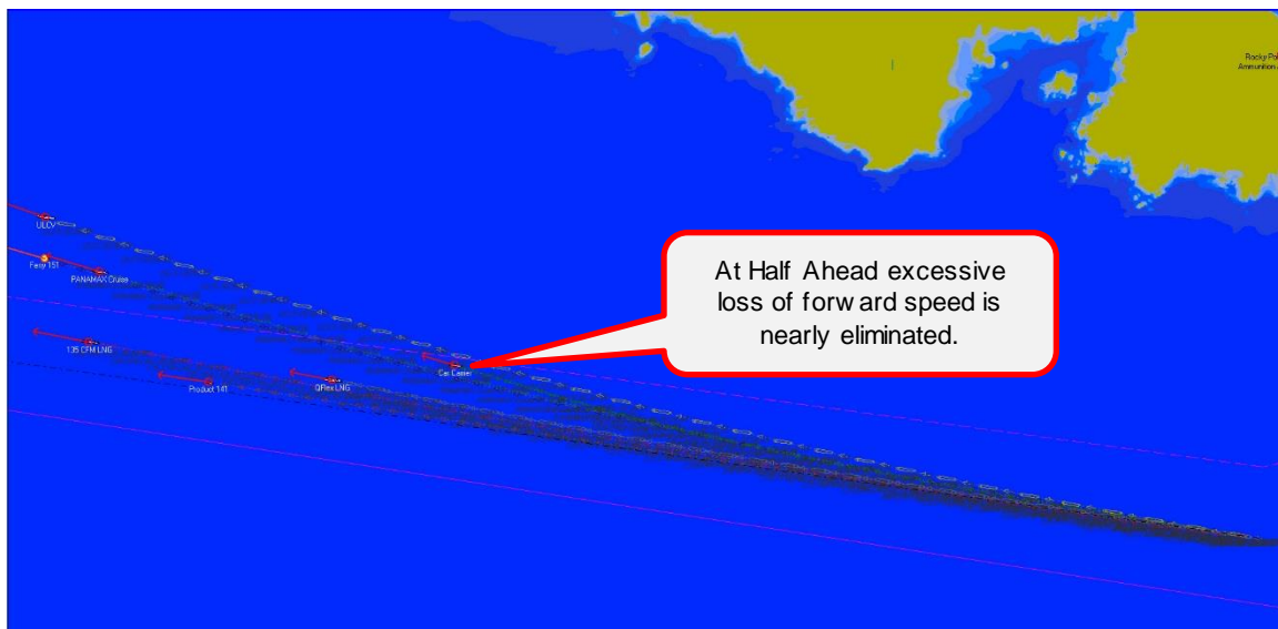
Figure 80: JDF TSS Heading Holding Test 13 Group 3 Wind 247° Half Ahead Track-plot
