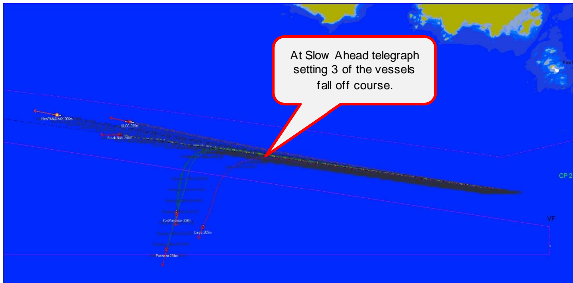
Figure 65: JDF TSS Heading Holding Test 10 Group 1 Wind 143° Slow Ahead Track-plot
