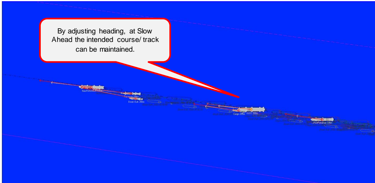
Figure 61: JDF TSS Heading Holding Test 9-1-Group 1 Wind 247° Heading and Course Graph
