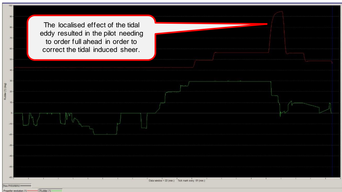
Figure 168: Propeller RPM, Test G1 T4_4 Neo-PANAMAX - Max Flood Wind 180@25
