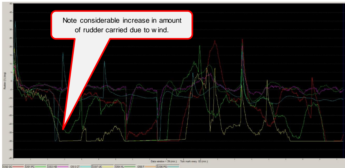
Figure 118: Test Group 1 Applied Rudder Graph: Downriver with Maximum Ebb - Wind 245° @30 knots
