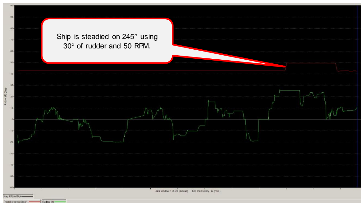
Figure 172: Rudder and RPM, Test G1 T8_4 Neo-PANAMAX - Max Ebb Wind 030@25
