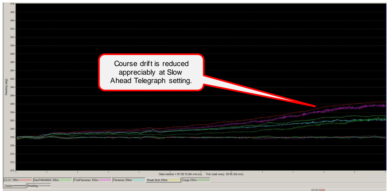
Figure 58: JDF TSS Heading Holding Test 9-Group 1 Wind 247° Heading and Course Graph
