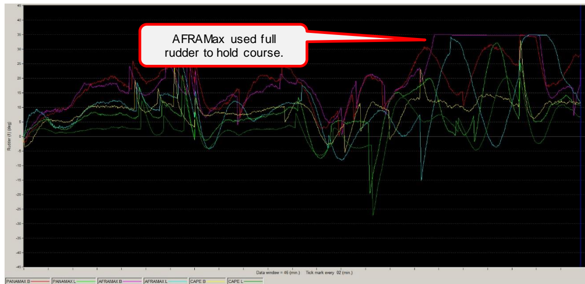
Figure 129: Test Group 2 Heading and Course Made Good: Upriver/Transit Speed 8 – Max Ebb/Wind 315° @30 knots
