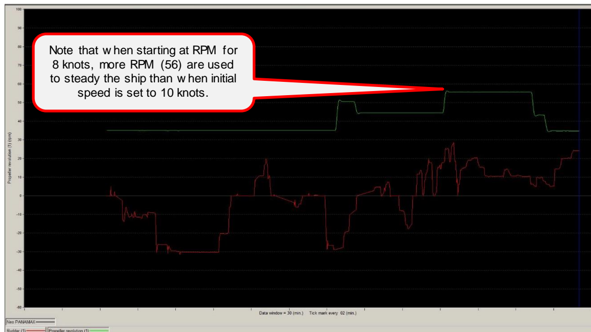
Figure 172: Rudder and RPM, Test G1 T8_4 Neo-PANAMAX - Max Ebb Wind 030@25
