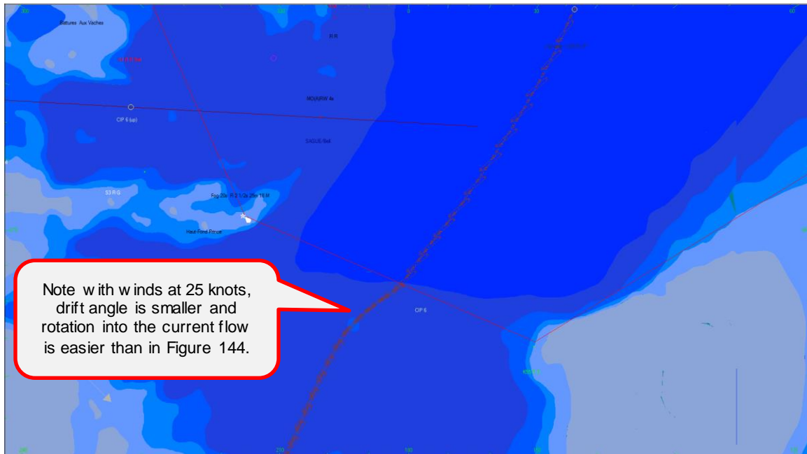
Figure 148: Trackplot Test G1 T10_2 – Upbound Maximum Ebb Wind 315 @ 25 Knots
