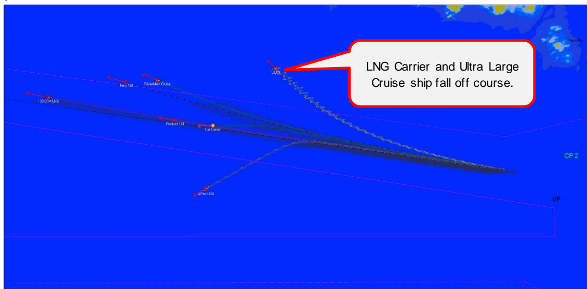
Figure 84: JDF TSS Heading Holding Test 10 Group 3 Wind 143° Dead Slow Ahead Track-plot
