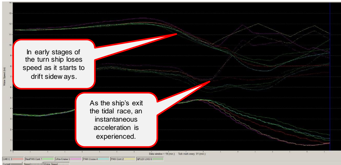
Figure 141: Exiting Tidal Race Instantaneous Acceleration: Test G1 T4 Speed Graph
