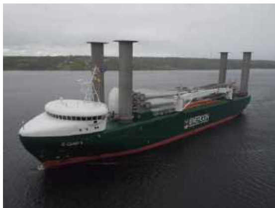
Flettner rotor on E Ship 1, source: IWSA
