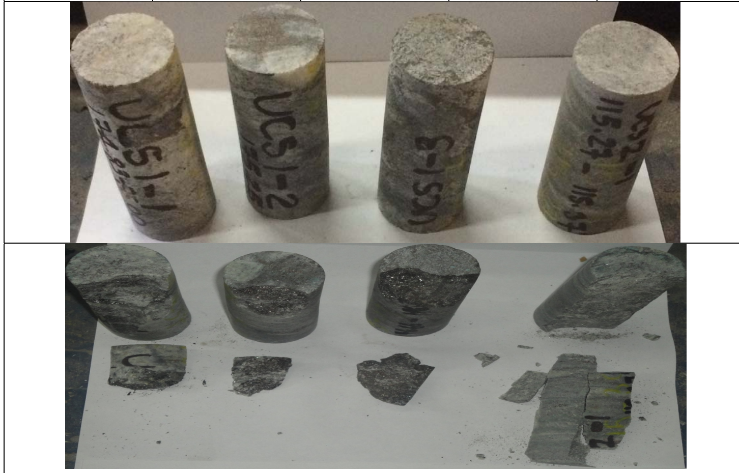
Figure 8-1: UCS samples before and after testing showing the general tensile splitting of cores.
