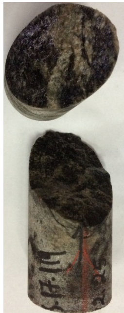
Figure 8-5: Typical ‘clean staining’ joints encountered within the host paragneiss rock formation.
