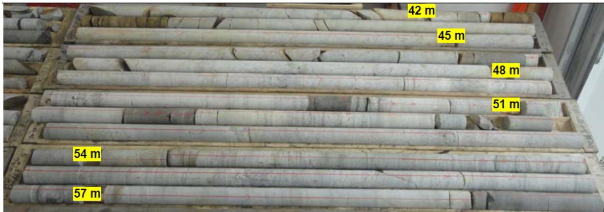
Figure 7-1: Example of rock core photos with recovery and RQD measurements (borehole TO-17-118).
