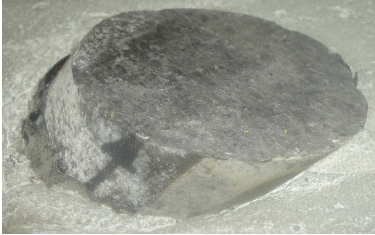
Figure 8-6: Typical smooth high rich graphite joint
