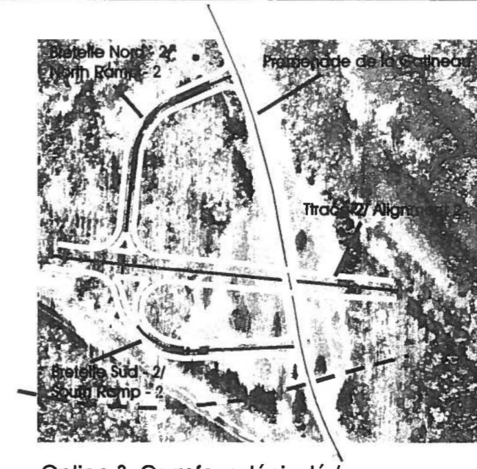
Option 3: Carrefour dénivelé / Grade separated interchange
