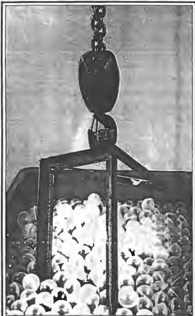
■ A demonstration model showing how metal objects can be dipped into tanks without having to move the Allplas Ball Blanket cover
